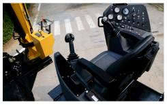
**THE OPERATOR'S STATION.** That is ergonomically designed with integrated joystick with fingertip buttons, switches and controls.
