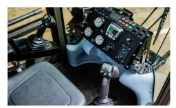
**THE OPERATOR'S STATION.** That is ergonomically designed and installed using integrated joystick with fingertip buttons, switches and waterproof controls.
