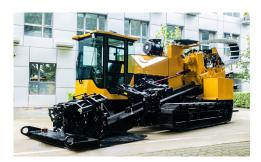
THE HIGH SPEED SEMI-AUTO ROD STAGER. Coupled with a high speed carriage at 42 m/min, it is a standard setting that enables faster drill rod coupling and improves work efficiency.
