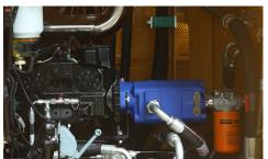
A SAUER-DANFOSS CLOSED-LOOP PISTON PUMP. That is utilized with merits of low energy consumption and high efficiency.
