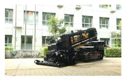
**THE FULLY AUTOMATIC DRILL ROD LOADER.** Maximizes the efficiency of the drill road exchange process, greatly improving the overall project efficiency.
